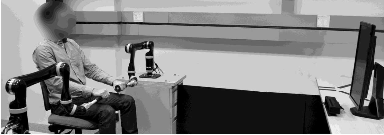
Figure 3. Experimental Setup. Participants moved the robotic devices while completing the reaching task (displayed in the computer monitor). In addition, a motion tracking camera was placed in front of the participant to monitor trunk compensation.
