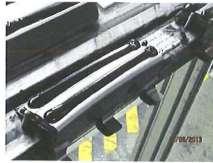
Figure 1. Example of a manually glued reinforcement plate. The applied glue stripes are not uniformly distributed along the plate.
